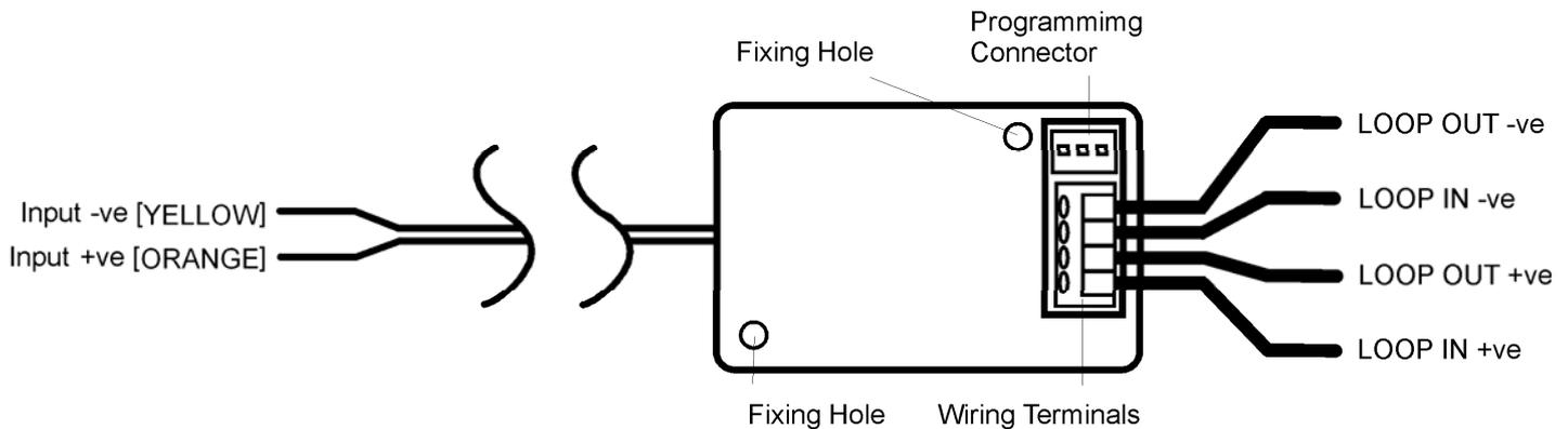
Fig 1 CHQ-SIM Wiring
