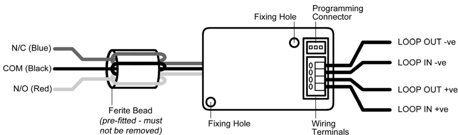
Fig 1 CHQ-SOM Wiring
