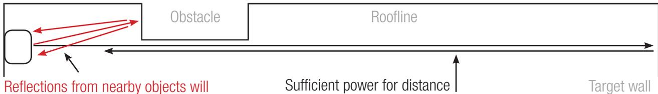
Reflections from nearby objects will limit the output power and prevent ability of the beam to cover the required distance
