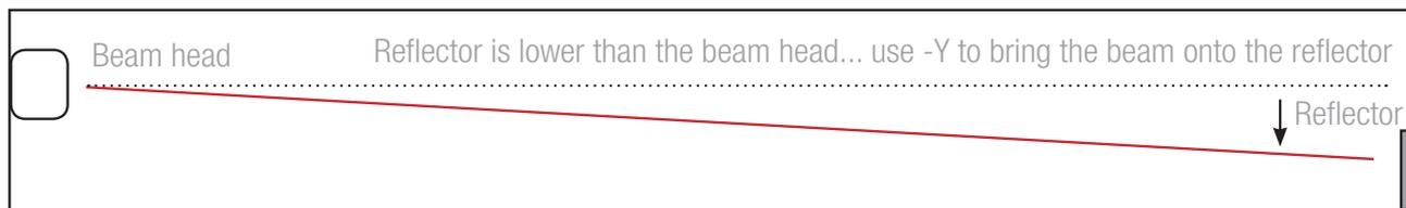
the firebeam can be moved on both X and Y axis to a maximum 5 degrees using the left (x-), right (x+), up (y+) and down (y-) keys. Looking at the reflector this will move the beam across the reflector. Holding the keys will quickly scroll through to your desired position, on release of the button the screen will revert to the actual beam position and can be seen stepping toward the requested position.
