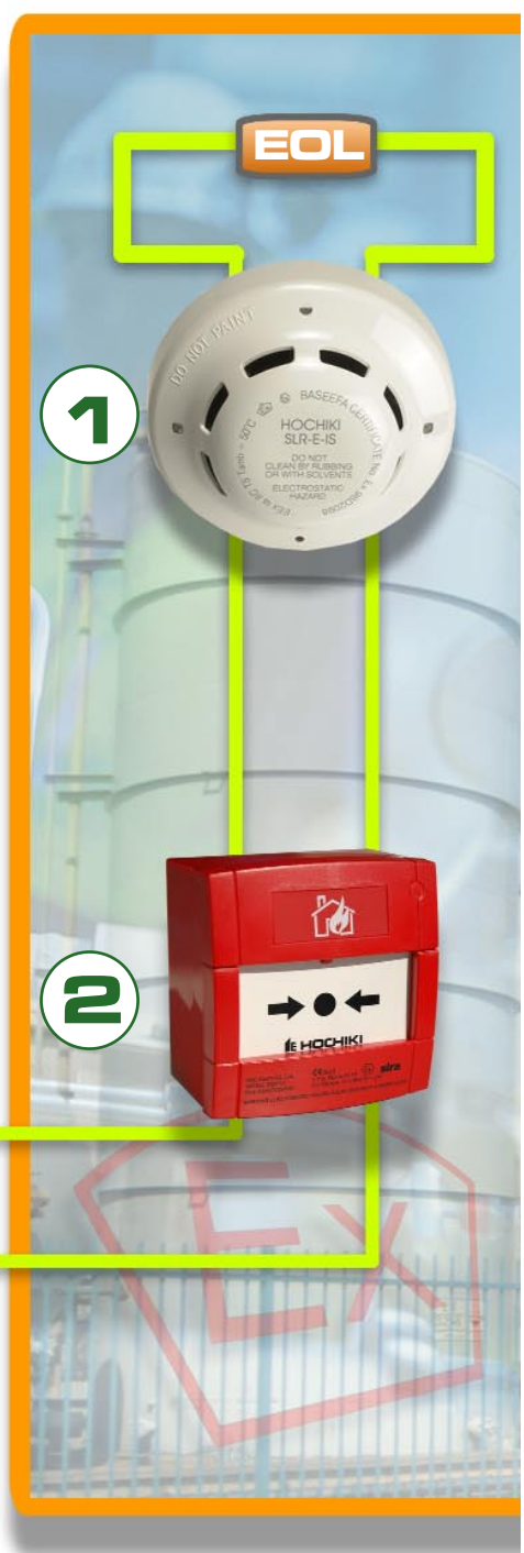
Zener Barrier (must be earthed) OR Galvanic Isolator
