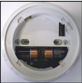
Picture 6 - primary and secondary batteries inserted
