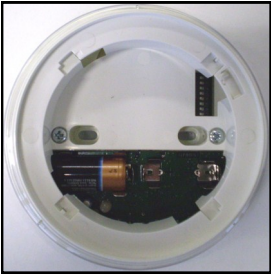
Picture 5 - secondary battery inserted
