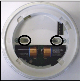
Picture 8 - position of the holes for screw's insertion
