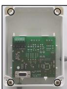
Picture 5 - wall fixing screw holes
