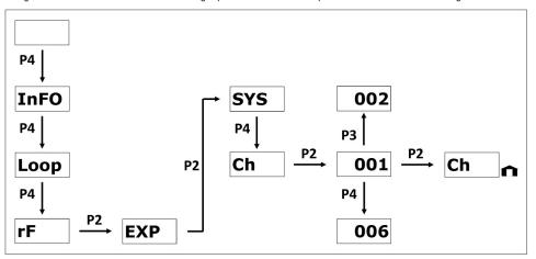
As can be seen, after channel selection, a little house icon appears on the lower right side of the display; this indicates the user that the translator's parameters have been changed
