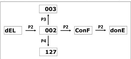
Bear in mind that this command deletes a device from the configuration of the translator, but not from the configuration of the main control panel: in this case control panel's configuration needs to be manually updated or the wireless system needs to be re-achieved by the control panel itself.
