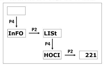
Dots cannot be visualized on the display, so, considering the above example, the 221 should be considered as 2.21.
