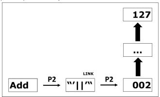
After the ADD command is performed, the translator waits the installer to trigger the linking of the child device by acting on the child device's "link-program switch" (see the specific installation manuals of these devices); during this phase, the LINK message is displayed and DL4 is switched on the translator; as a matter of fact the translator is waiting to achieve, in its configuration, the child device.
