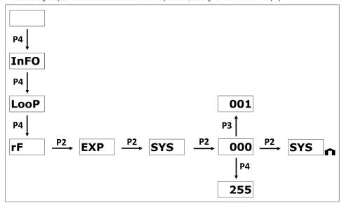
As can be seen, after the selection of the system identifier, a little house icon appears on the lower right side of the display; this indicates the user that the translator's parameters have been changed
