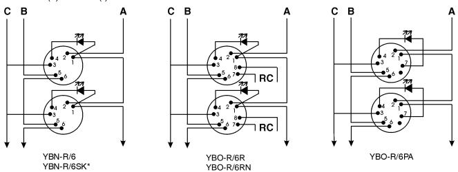
RC Relay Contacts - a flying lead on either terminal 7 or 8 selects either N/C or N/O (supplied as N/C)
